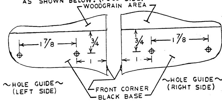
2) MOUNT TRAY SUPPORTS WITH SCREWS AND WASHERS PROVIDED AS SHOWN BELOW:
